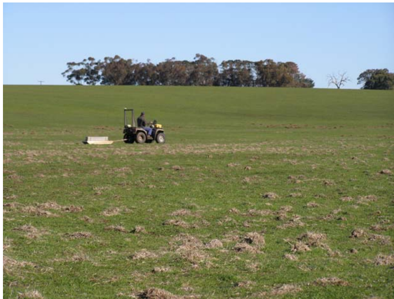
Figure 4-1 Geophysical Survey – Geonics EM38 device trailing behind a Bombardier ATV.
