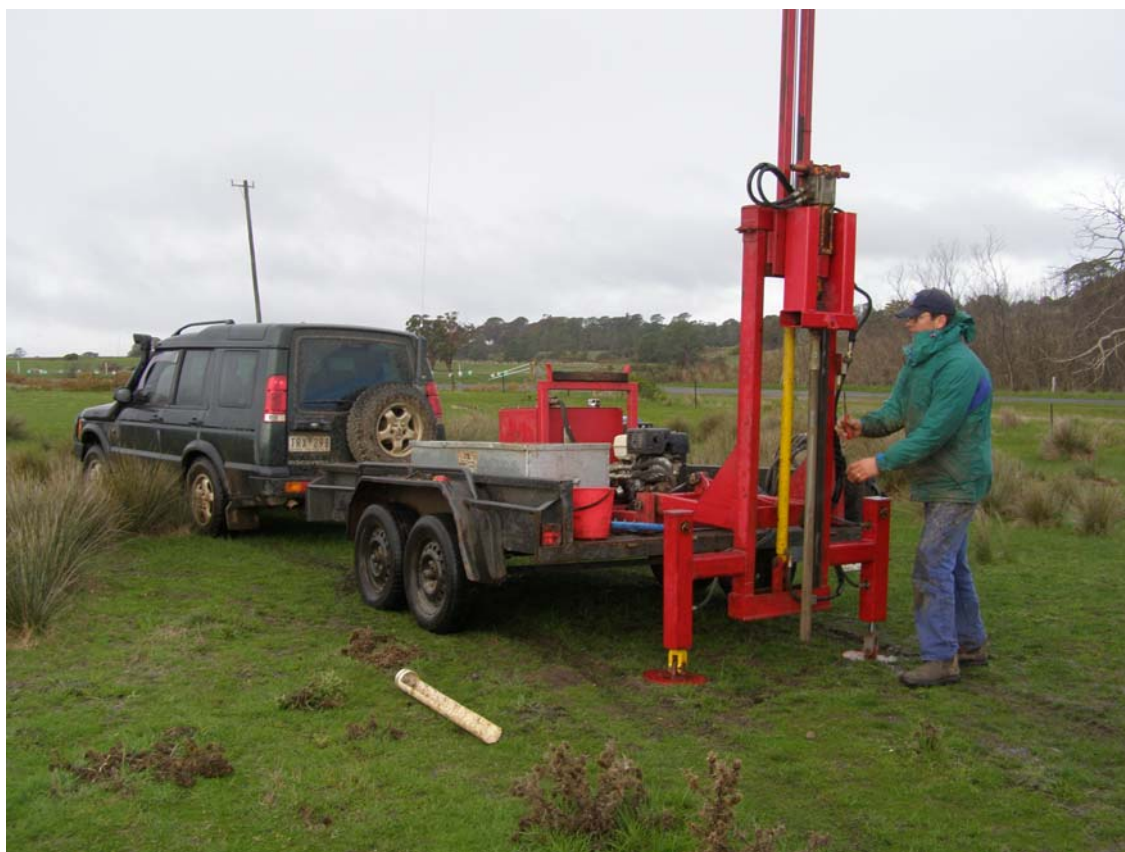
Figure 4-2 Hydraulic Corer - used to sample soil to approximate depth of one metre.
