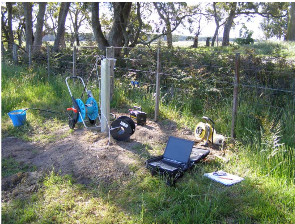
Figure 4-5 Aquifer recovery testing – Mount Mercer, MM3.
