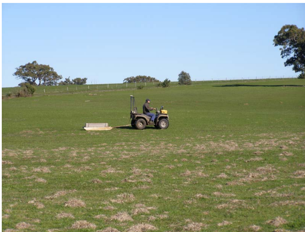
Figure 4-1 Geophysical Survey – Geonics EM38 device training behind a Bombardier ATV.
