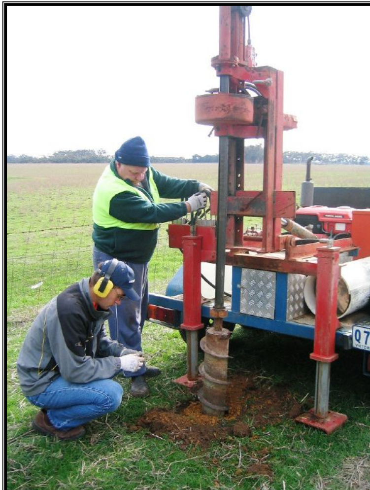
Figure 20 A trailer-mounted Pengo-type drill was used for the extraction of intact soil cores (Photograph S McConachy).
