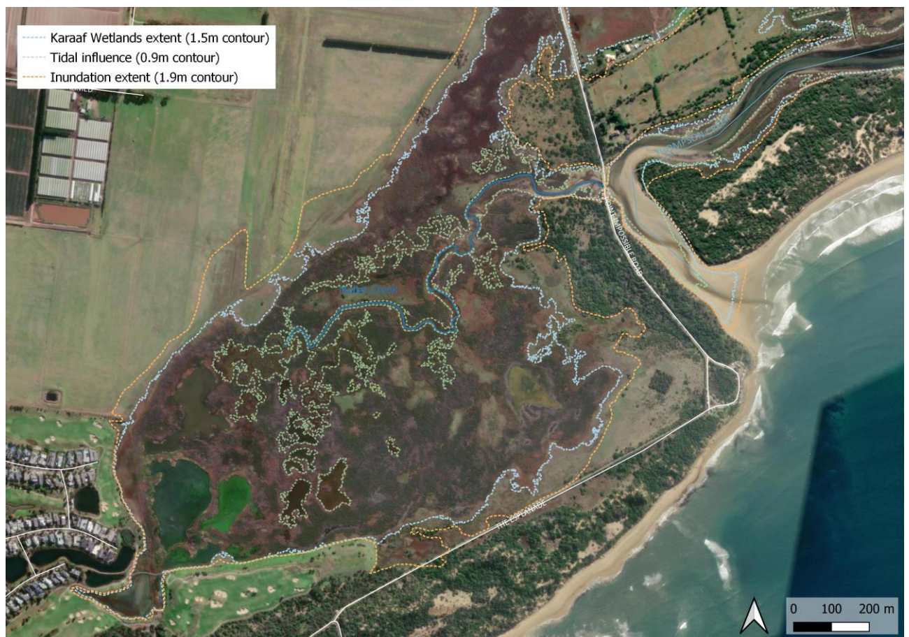
Figure 17 Comparison of coastal water levels and elevations across the Karaaf wetlands
